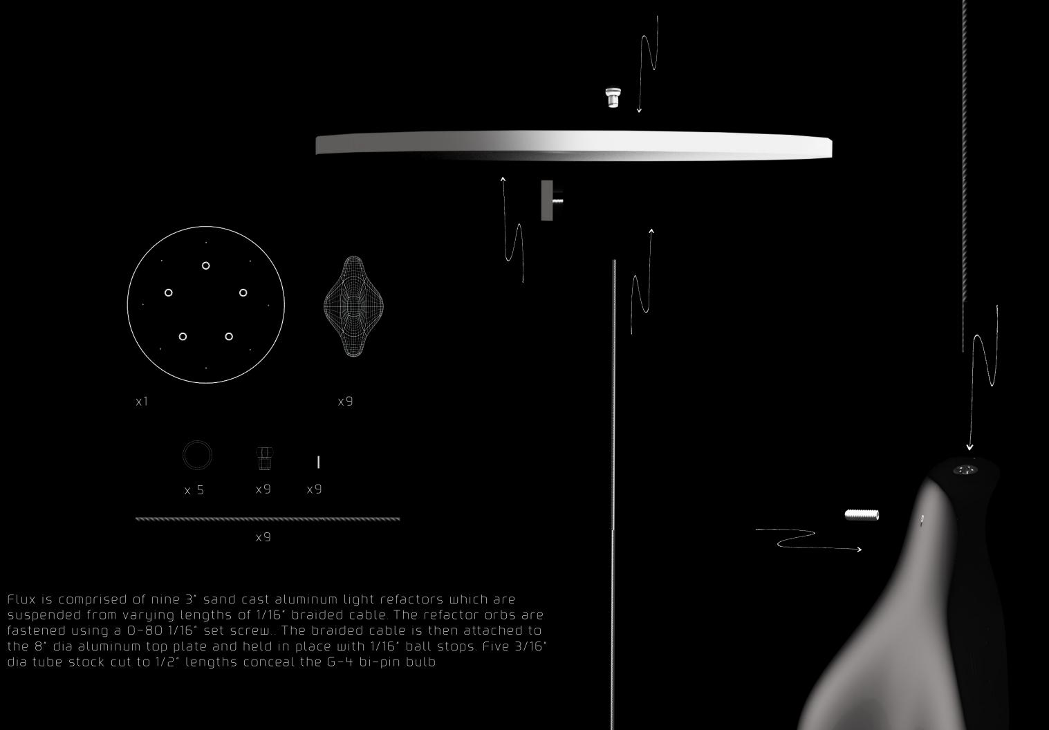
Sand cast 60/61 alloy aluminum refactor form
