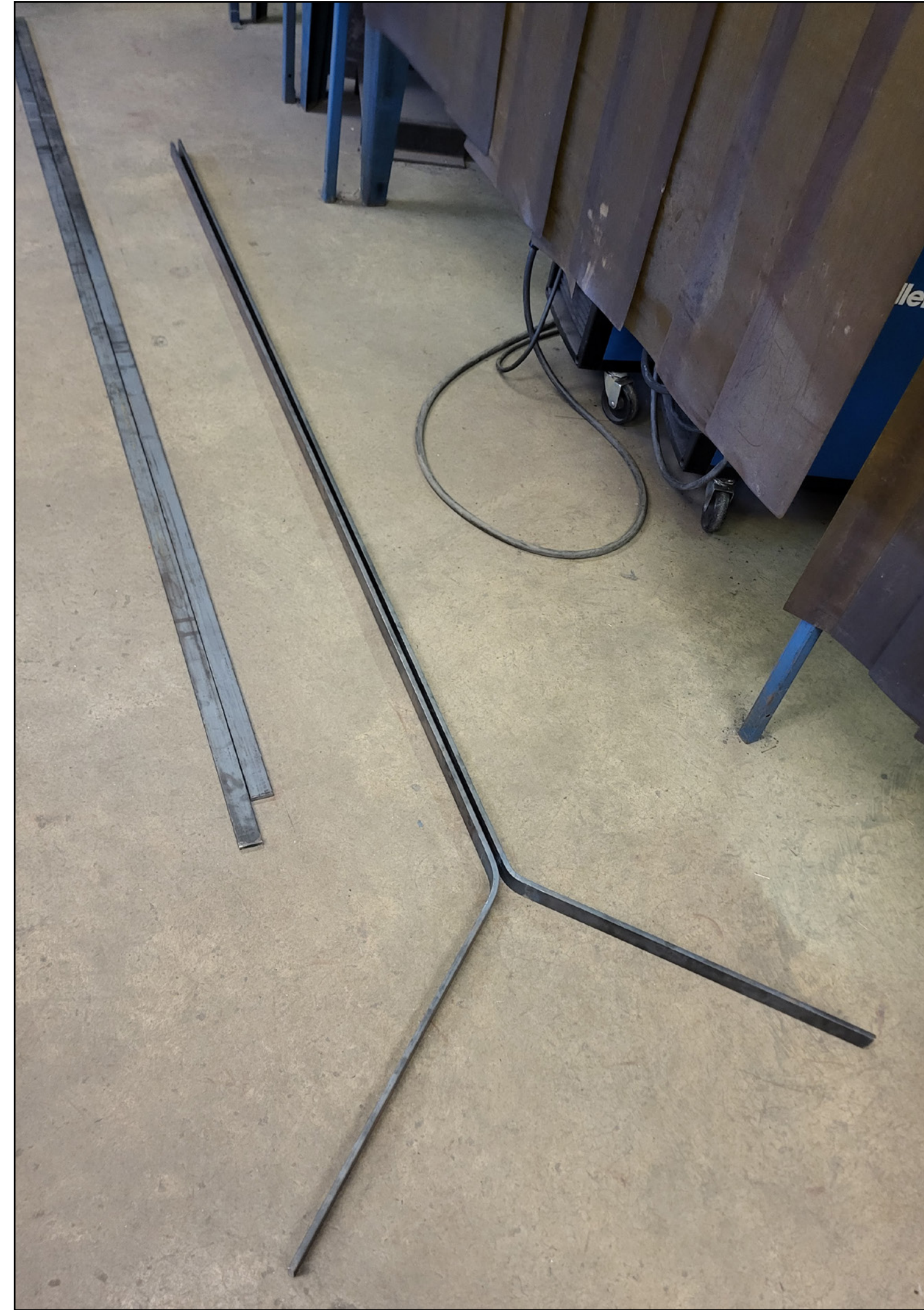
-3/8" STEEL HEATED USING AN OXY ACETYLENE TORCH AND BENT TO SHAPE ON A JIG
