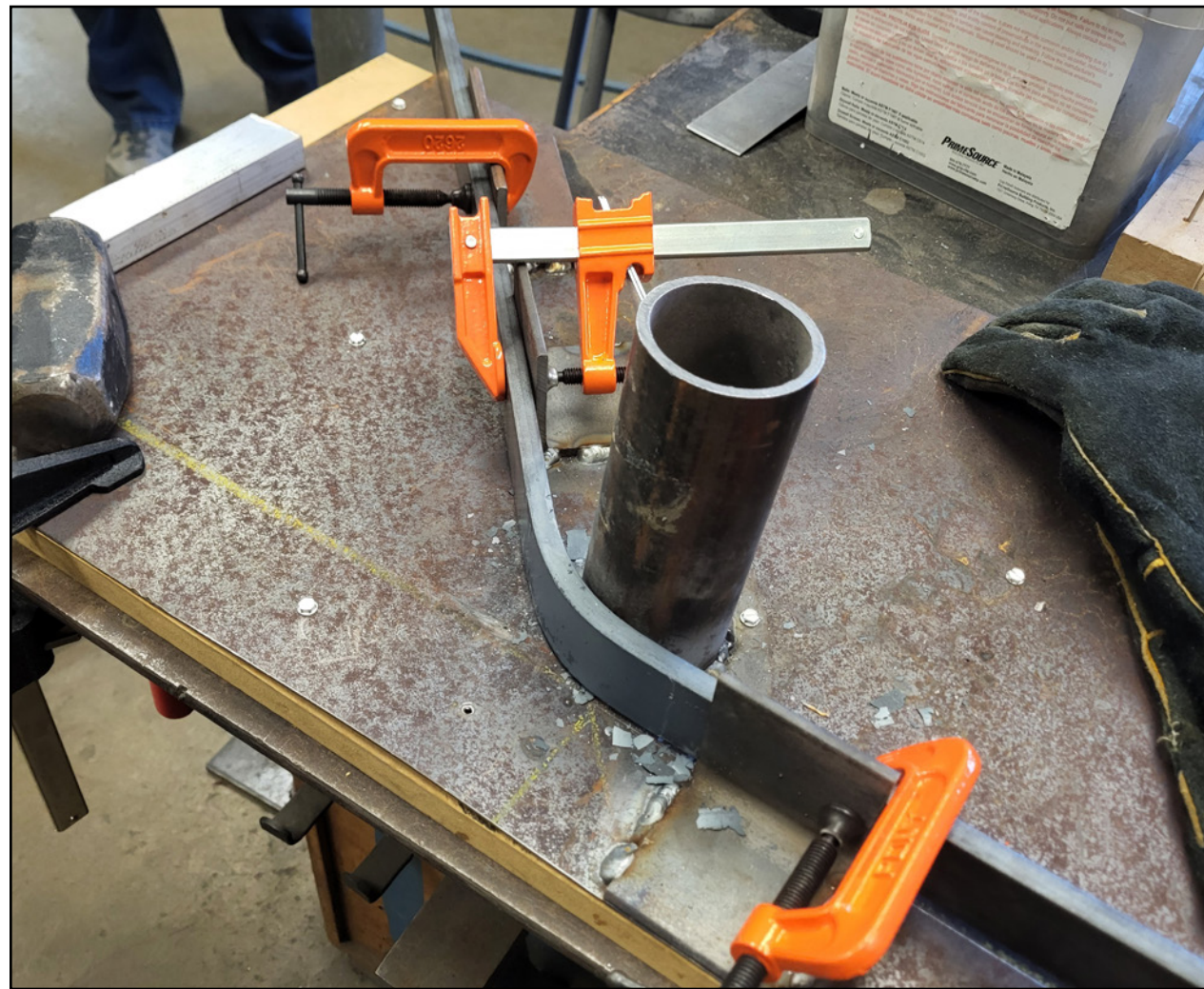
-3/8" STEEL HEATED USING AN OXY ACETYLENE TORCH AND BENT TO SHAPE ON A JIG
