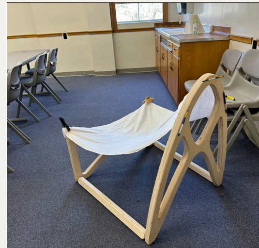
making pattern for suede sling to ensure proper draping & minimize error
