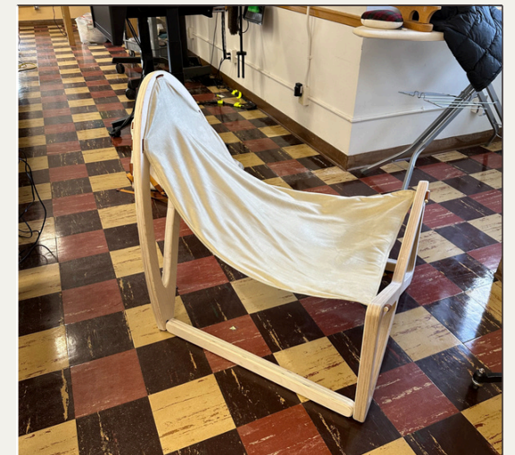
sewn sling. double layered and triple stitched
