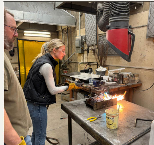
using AAE metal shop to patina steel rods
