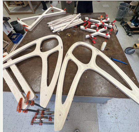
cnc piece gluing to reach desired thickness
