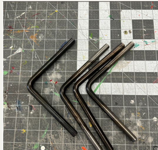
patina steel rods to achieve desired steel finish
