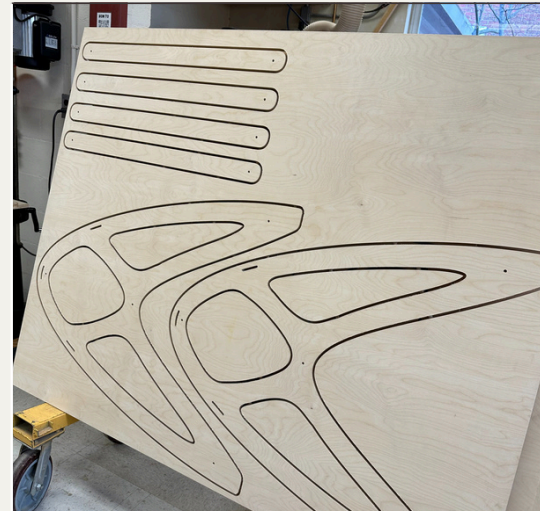
after finalizing cad files, cnc pieces were cut
